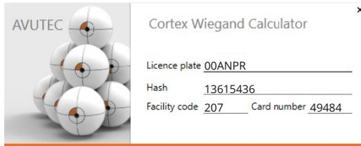
The Gatekeeper converts a number plate into a Wiegand output message, like a card reader or biometric reader. AVUTEC offers the Cortex Wiegand Calculator to convert number plates into a standard Wiegand card number which is needed to represent these number plates. The Cortex Wiegand Calculator can be found at [AVUTEC.com/support](http://AVUTEC.com/support) and is available as a license-free Windows application at your AVUTEC dealer.
